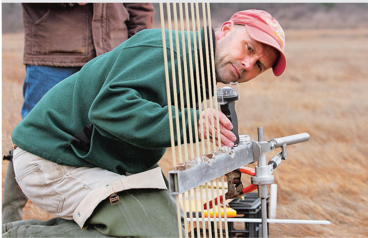
Scientist Kenny Raposa uses a surface elevation table (SET) device to gauge growth at Nag Marsh on Prudence Island. His goal is to determine whether marshes are gaining altitude, key to survival against rising seas. [THE PROVIDENCE JOURNAL/BOB BREIDENBACH]
