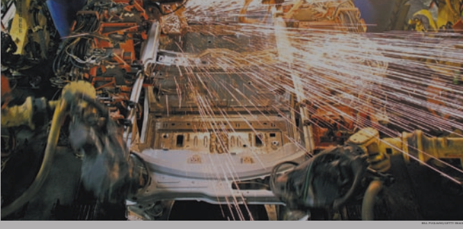
Robot arms weld a car body at a General Motors plant in Lansing, Mich., in 2010.
